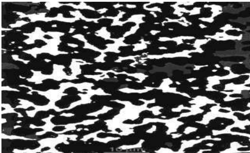
Fig. 1. Gray-scale digitized microscope image of a three-phase boron carbide/aluminum composite: white region is Al phase, blackregion is B_4C phase, and gray region is Al_4BC phase. The B_4C and Al phases are the dominant ones.
